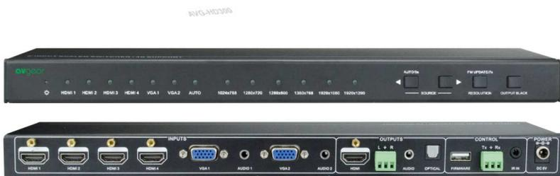
The AVG-DSS61 is a compact 6x1 mini scaler switcher with 6 video inputs (4 HDMI, 2 VGA), 2 auxiliary audio inputs (switched following VGA), 1 HDMI output and 3 audio outputs (1 dual-mono analog audio, 1 3.5mm stereo audio, 1 optical audio).
